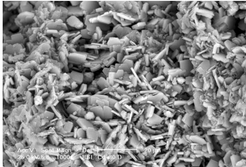
Figure 1. SEM image of zeolitic rock treated with 0.002 M \text{Cd}(\text{NO}_3)_2 solution for 48 h at 303 K.
